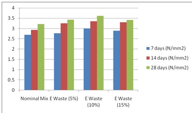
**Fig 7 Flexural Strength Test Results**
