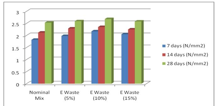
**Fig 6 Split Tensile Strength Test**
